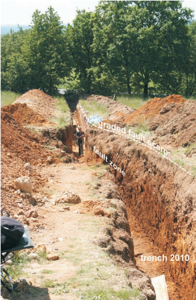
Fig. 12: Field impression the the paleoseismological trench across the MLF fault zone made by ŠTĚPANČÍKOVÁ & FISCHER (2012). The discontinuity of the slope coincides with a fault zone displayed in the trench.
